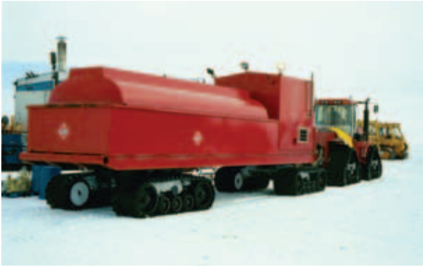
Figure 2.122. Fueling vehicle on rubber tracks pulled by a rubber tracked tractor.
