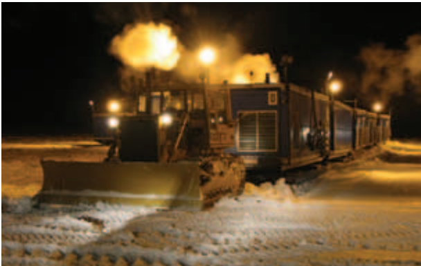
Figure 2.123. Dozer pulling a camp train. The steel tracked dozers are being phased out and replaced by the rubber-tracked tractors.
