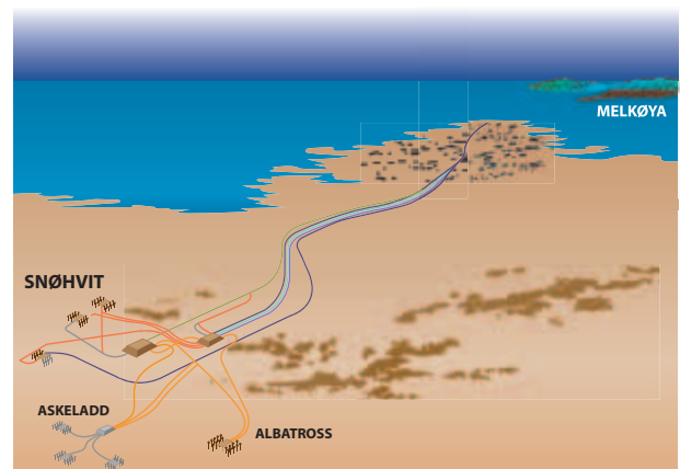
Figure 2.141. Schematic of sub-sea installations and pipelines of the Snøhvit field (courtesy of Statoil ASA).
