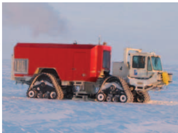
Figure 2.35. Modern tracked vibrator with the plate down.
