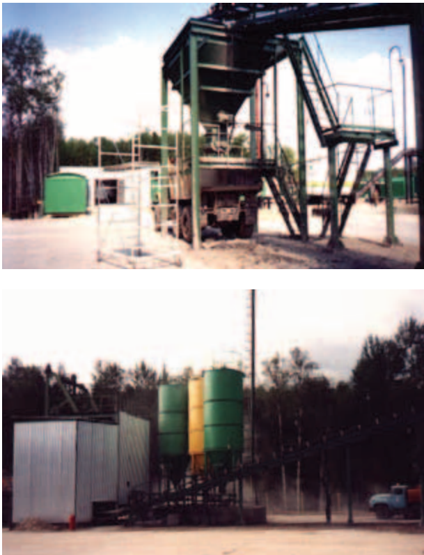
Figure 2.121. The drilling mud treatment facility at the OAO Yuganskneftegas test site for storing drilling mud and oil-contaminated soils.
