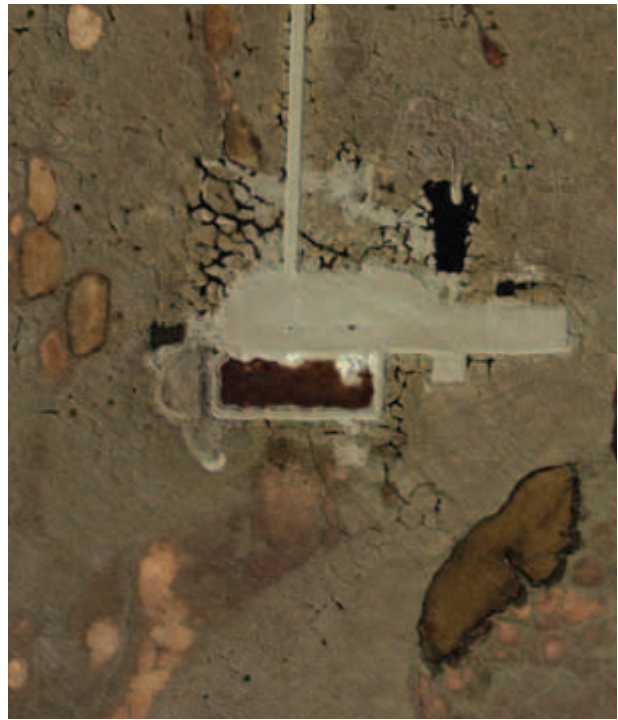
Figure 2.119. Old exploration drill site with gravel pad and road.
