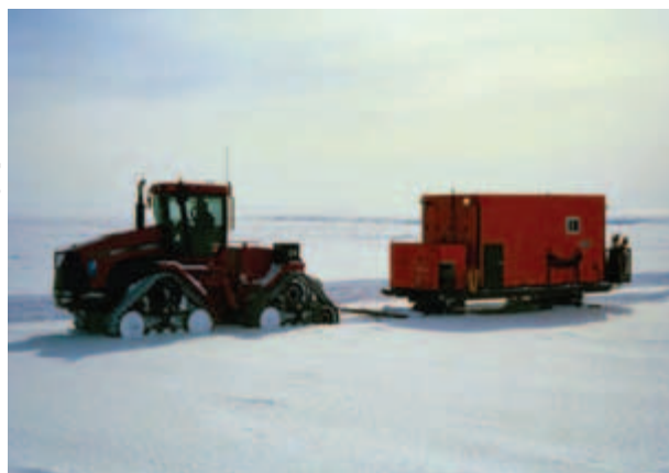
Figure 2.34. Prime mover on rubber tracks pulling a trailer on skids.
