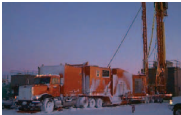
Figure 2.134. Typical coil tubing unit.
