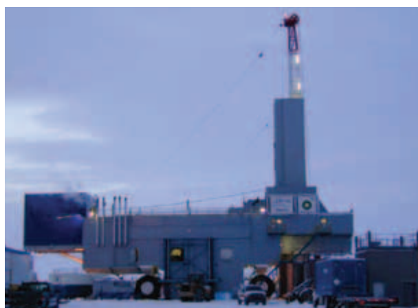
Figure 2.135. Typical coiled tubing drilling rig.
