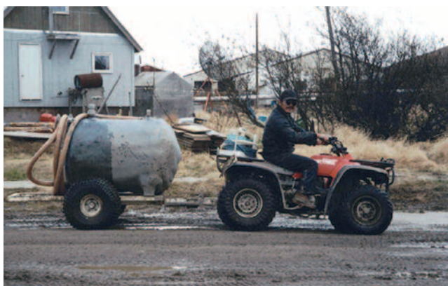
Fig. 15.11. All-terrain vehicle water haul system, Mekoryuk, Alaska (photo by Mark Baron).
