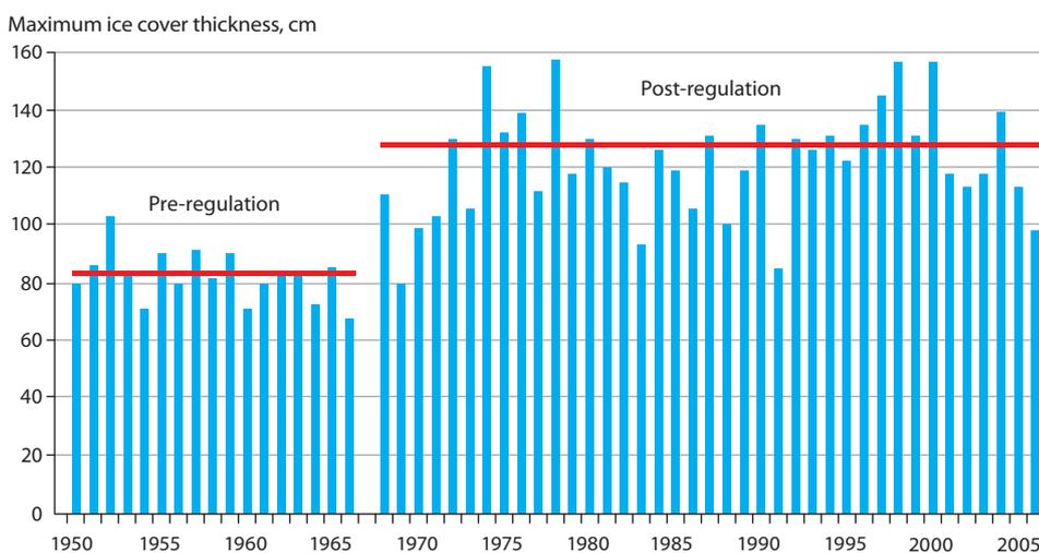
Figure 6.8. Step-change in maximum ice-cover thickness at the Tuoy-Haya station before regulation (river channel, 1951 to 1967) and after regulation (nearshore zone of Vilyuiskoye reservoir, 1969 to 2007). Data sourced from the State Hydrological Institute, St. Petersburg, Russia.
