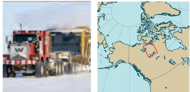
Figure 6.22. Example of large loads transported on the Tibbitt to Contwoyto Winter Road in northern Canada, which is composed of many long reaches across frozen lakes and rivers. Photo courtesy of Joint Venture Management Committee, partnership between DeBeers Canada, Inc.; BHP Billiton, Ltd; and Diavik Diamond Mines, Inc.
