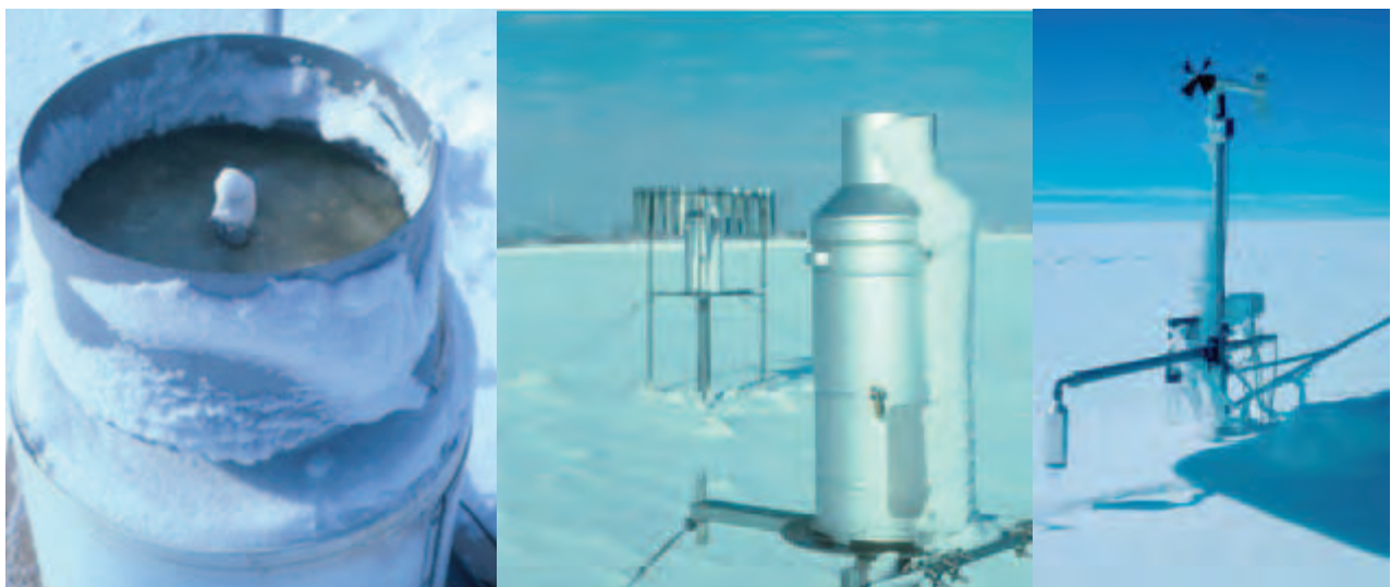
Figure 11.16. Conditions can make quality control challenging for solid precipitation measurement in the Arctic. Photos courtesy of B. Goodison, World Meteorological Organization.
