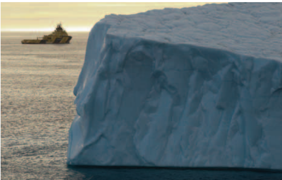
Figure 10.8. Icebergs constitute a hazard to Arctic offshore oil operations. A tug boat stands by to tug an iceberg away from a drilling area. Photo: Will Rose / Greenpeace.
