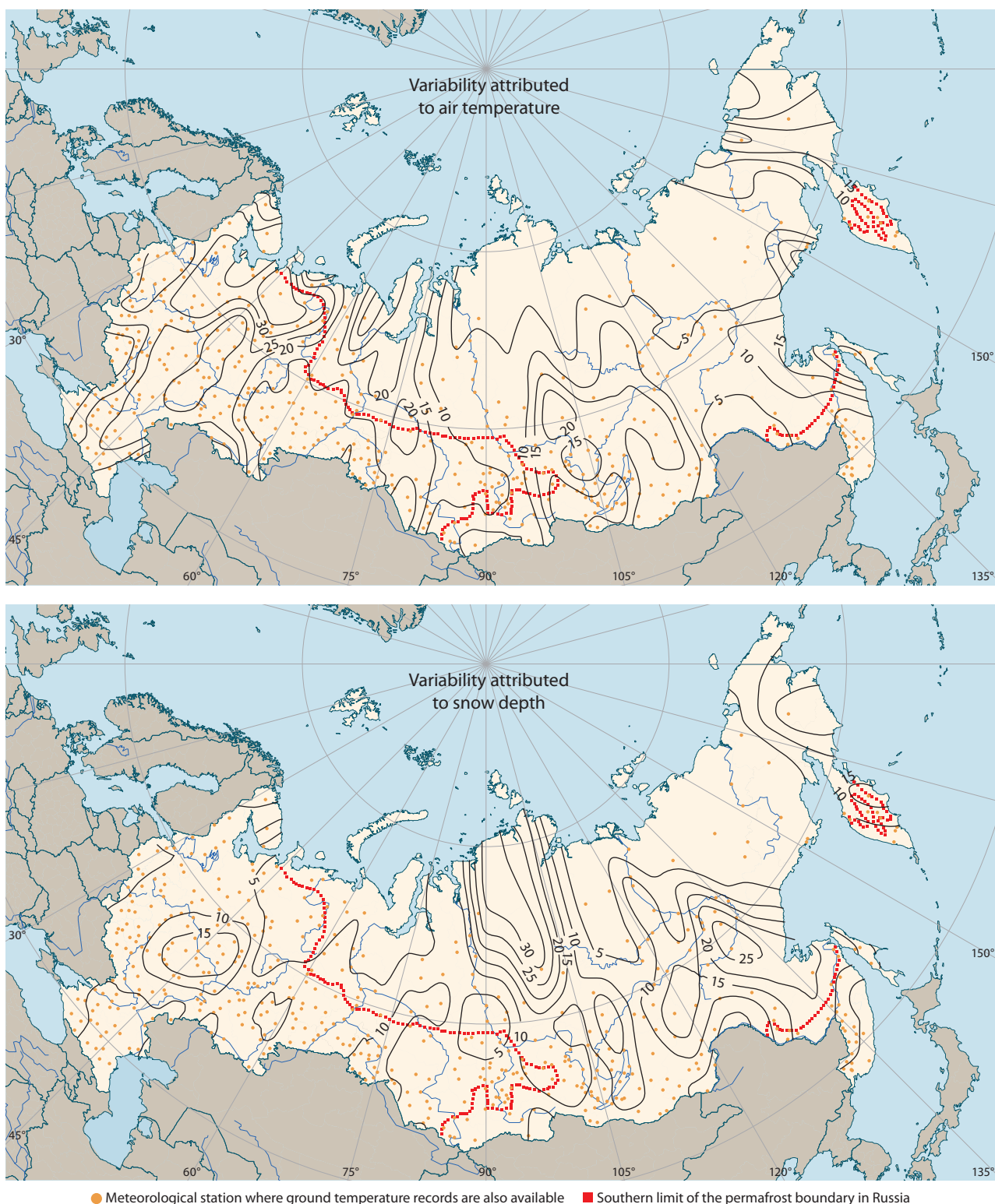
Figure 4.14 Percentage of total ground temperature variability attributed to air temperature (upper) and snow depth (lower) (Anisimov and Sherstukov, 2016).
