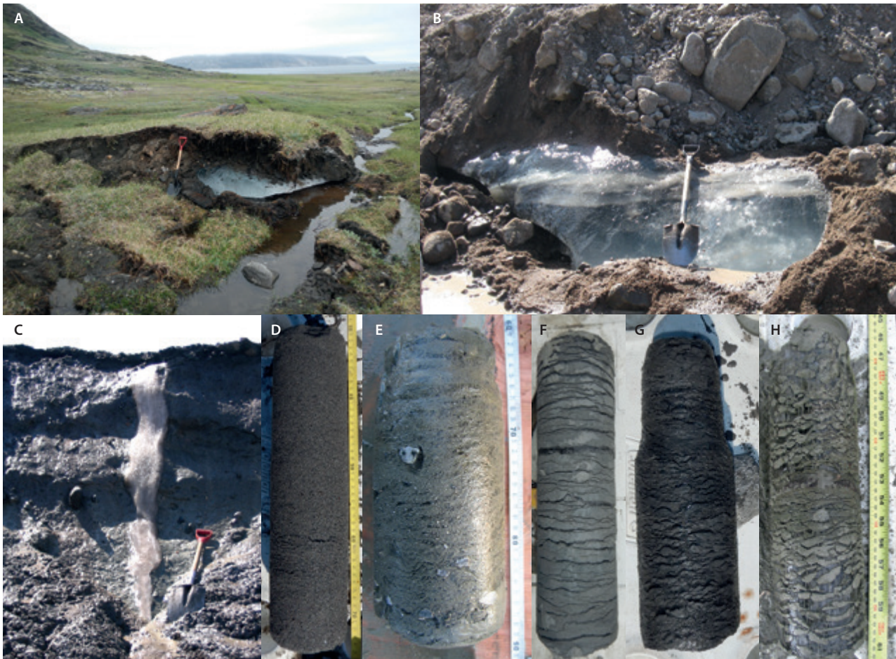
Figure 10.6 Examples of types of massive ground ice (panels A–C) and ground cryostructures (panels D–H) encountered in permafrost over the BBDS region: (A) Massive ground ice mound – a frost blister, (B) Buried massive glacier ice, (C) An ice wedge, (D) Structureless – porous non-visible ice, (E) Lenticular – microlenticular segregated ice lenses, (F) Layered – wavy, segregated ice lenses, (G) Irregular reticulate – segregated ice lenses, and (H) Suspended/reticulate – segregated ice lenses (photos by E. L’Hérault).
