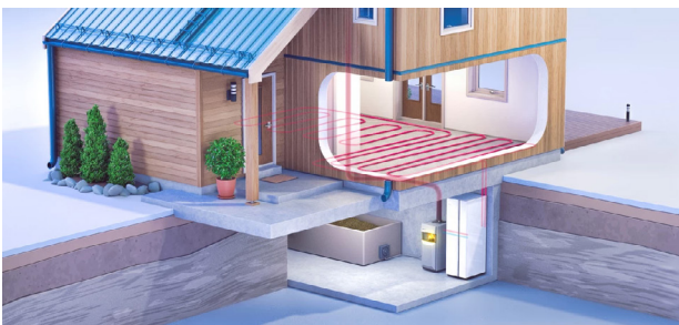
Figure 4: Water-borne heat in a residential building with a wood log/pellet boiler in the basement. Image credit: Enova.
