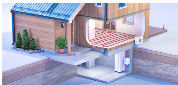
Figure 5: House with heat pump and water-borne heat distribution. Image credit: Enova.
