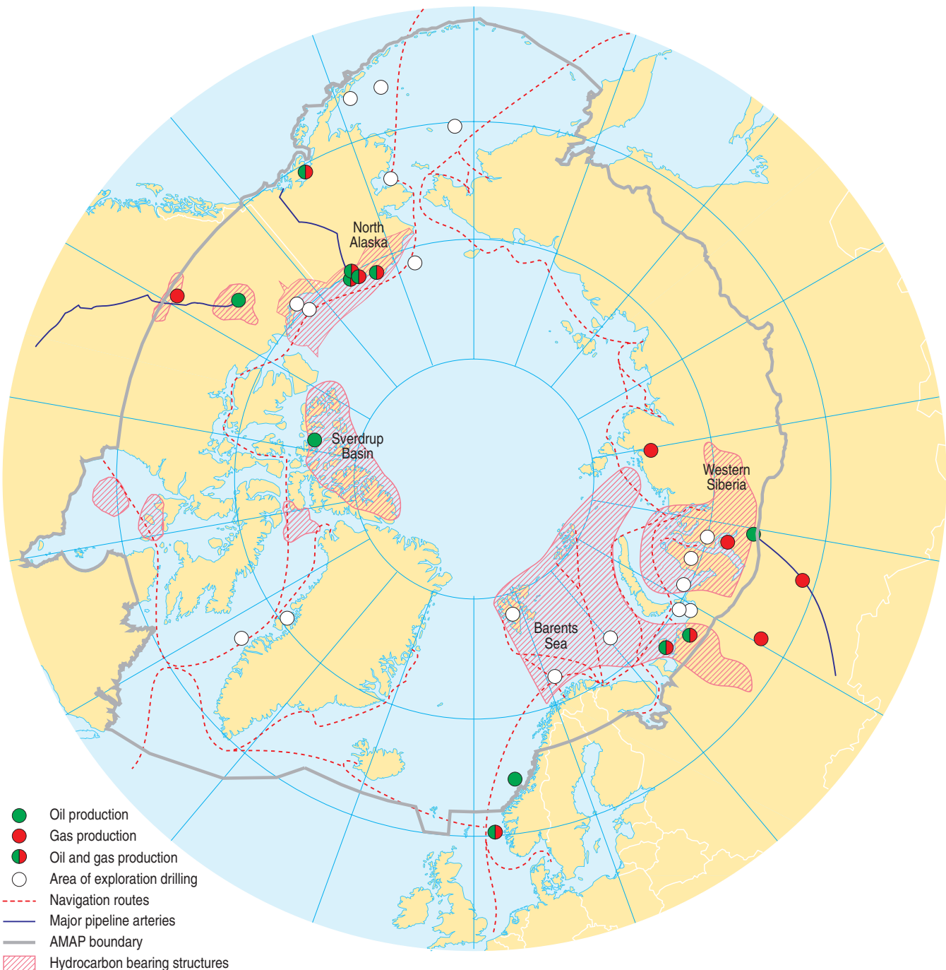
Figure 10-1. Major areas of oil and gas development and potential development in the Arctic, and major shipping routes and possible new routes through Arctic waters.
